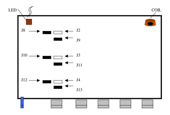
To allow a loop-output, the J2, J3 and J4 pins must be open on both the top and the bottom boards. Again, the outputs will be overdriven if there is no local monitor connected to the input when the termination is disabled. This may cause serious problems to the display device.
